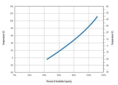
E. C.A. (Cranking Amps) - the discharge load in amperes which a new, fully charged battery can maintain for 30 seconds at 32°F (0°C) at a voltage above
