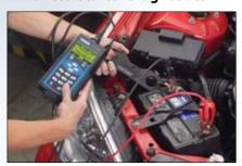
Using the optional Amp Clamp provides an enhanced level of diagnostics beyond just starter voltage drop. The EXP starter diagnostics include starter amps draw, voltage drop, start time, and starter circuit resistance resulting in more accurate results.
