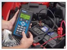
For Advanced Alternator Diagnostics the EXP uses superior DSP capability to digitize the measured alternator output voltage and evaluate the spectral content of the signal. This digitized signal allows the EXP to combine pattern recognition with the amplitude level of the AC signal for improved accuracy and identification of open or shorted diodes and open phase conditions, (multiple diode failure or winding problems).
