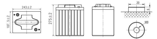
Note:Terminal Torque Values in-Ib(Nm):97.28-130.0(11-14.7)
