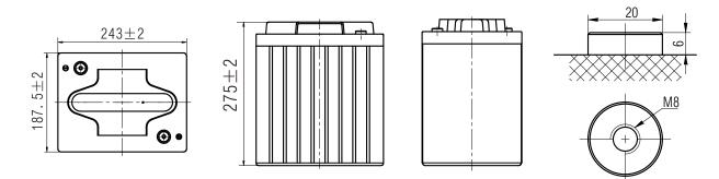
Note:Terminal Torque Values in-Ib(Nm):97.28-130.0(11-14.7)
